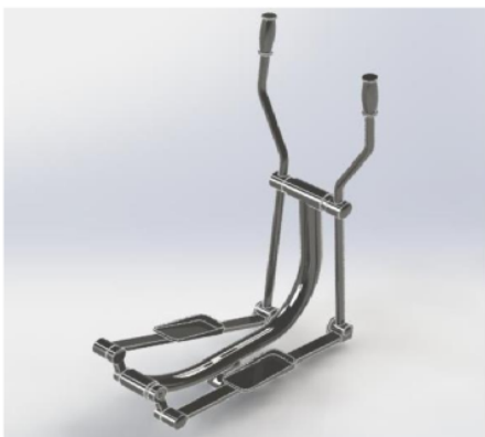
Gambar 2. Desain 3D alat elliptical trainer outdoor
