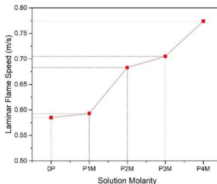
Figure 4. Graph of diffusion combustion flame speed before and after purification with 1M, 2M, 3M, and 4M CaO molarities.
