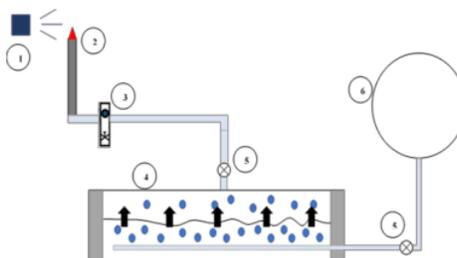
Figure 2. Schematic of biogas purification and combustion
