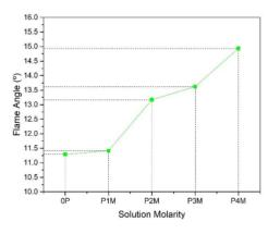
Figure 6. Flame Angle diffusion on combustion before and after purification with 1M, 2M, 3M, and 4M CaO molarities.
