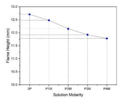
Figure 5. Biogas flame height in diffusion combustion before and after purification with 1M, 2M, 3M, and 4M CaO molarities.
