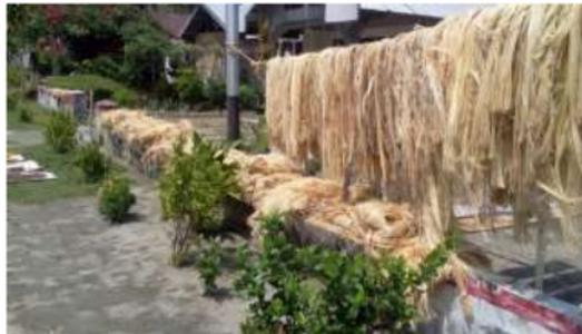
Gambar 4. Serat Abaca proses pengeringan, minimalisasi kadar air.
