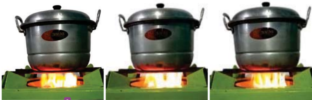
9 FIGURE 6. Flame stability of the briquette stove using an adjuster.
