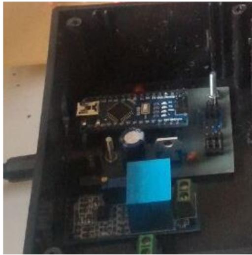
Figure 7. System Circuit with Arduino Nano, Proximity Sensor, Power Supply, and Buzzer
