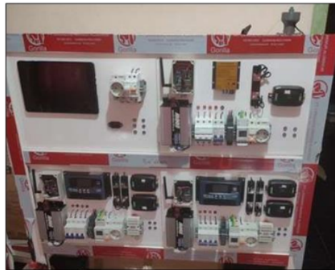
Gambar 3. Alat sistem monitoring PLTS berbasis Smartphone
