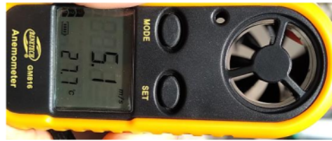
FIGURE 4. Wind speed measurement with Anemometer
