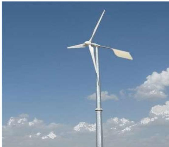
**Gambar 2.12 Turbin angin sumbu horizontal**
