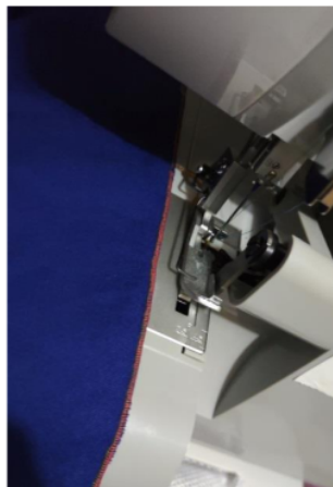
Figure 13. The results of the work using an edge sewing machine
