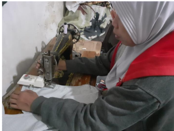
Figure 8. Manual buttonhole process with the production partner's single machine
