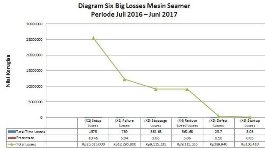
Gambar 10 : Diagram Pareto Sig Big Losses Mesin Seamer
